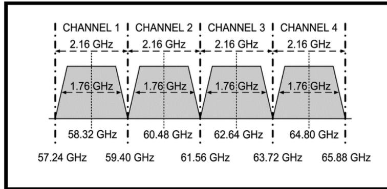
Figure 3: Channelling arrangement of the 60 GHz Band
