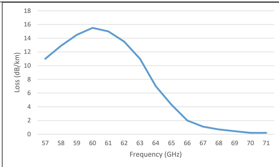
Figure 1: Graph showing high loss between 57 GHz to 66 GHz due to oxygen absorption from rain<sup>[HSN2]</sup>
