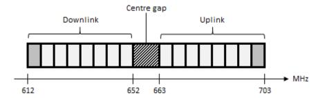
Figure 2: 600 MHz Band Plan for 470-703 MHz Band
