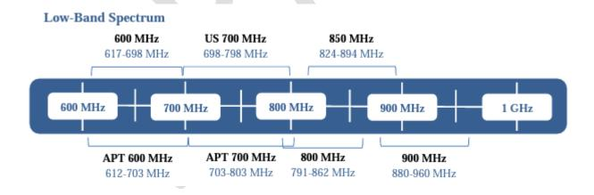
Figure 1: Low- Band and Mid-Band frequency bands that are used for Cellular Mobile Services globally
