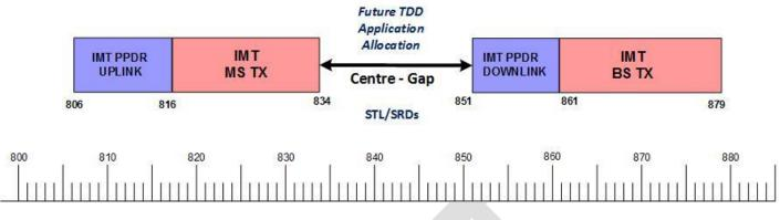
Figure A-1: 800 MHz IMT Channel Plan
