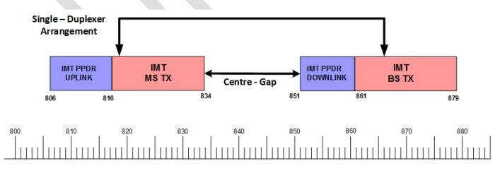
Figure 1: FDD Mode Single-Duplexer Frequency Arrangement
