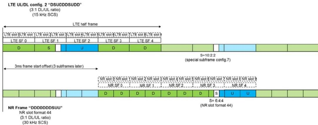
**Figure 4: Variant 2 - Synchronised operation of 5G-NR ("DDDDDDDSUU" frame) and LTE-TDD ("DSUDD" frame)**
