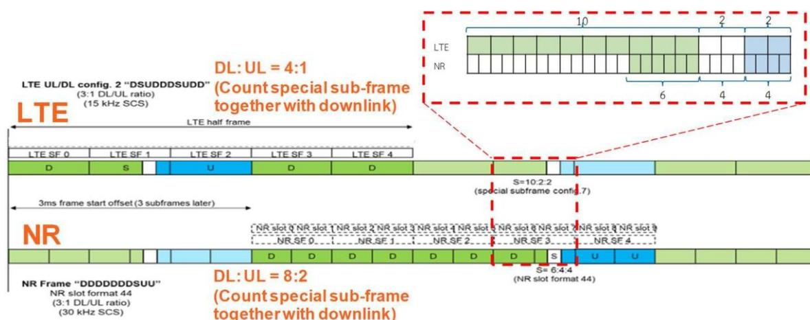
**Figure 5: Example of LTE and NR Frame Structure Configurations (Source: ECC Report 296)**
