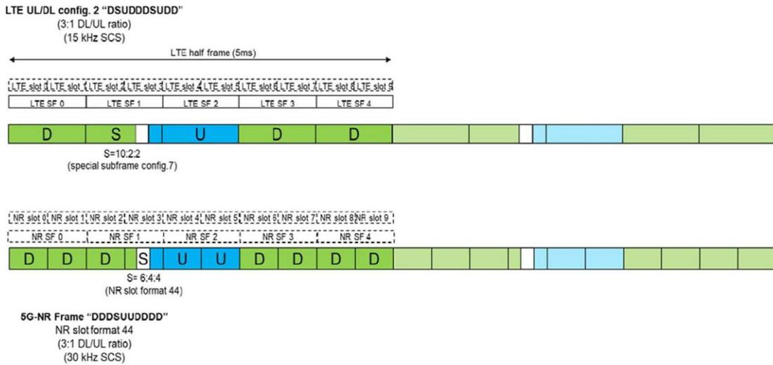
**Figure 3: Variant 1 - Synchronised operation of 5G-NR ("DDDSUDDDD" frame) and LTE-TDD ("DSUDD" frame)**
