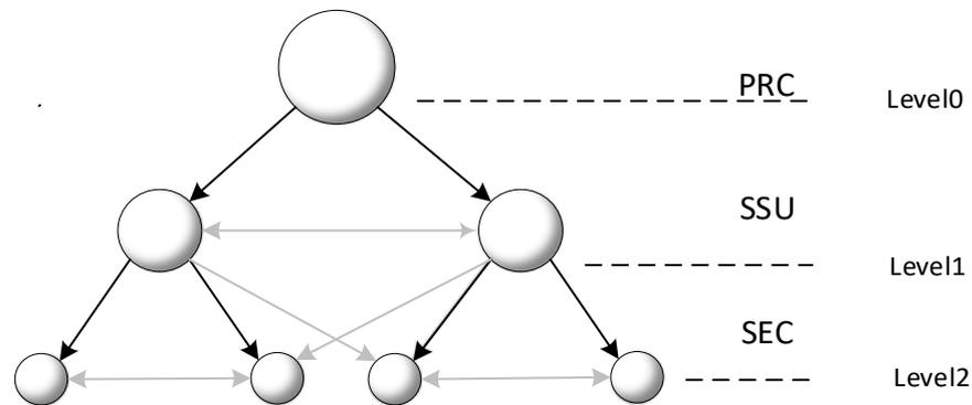
Figure 5.3 Hierarchical Master-Slave Synchronization
