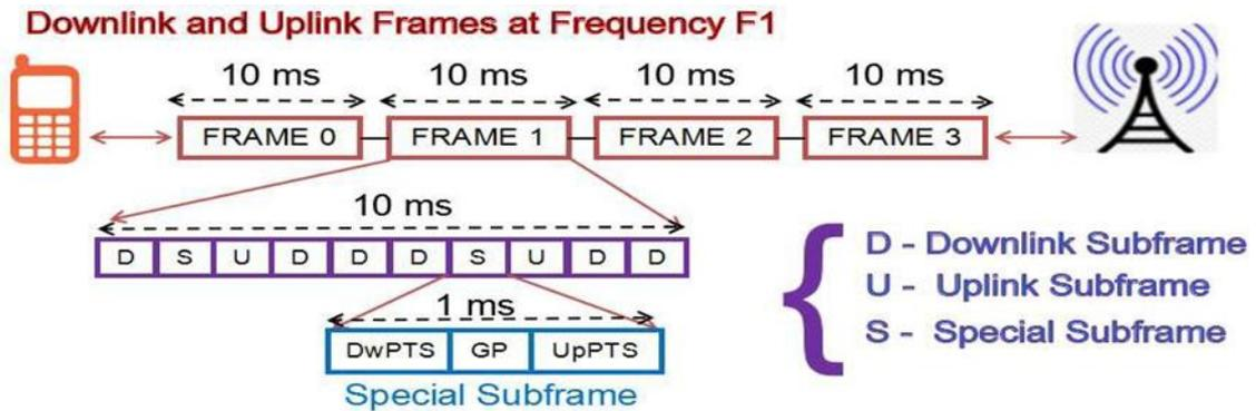
**Figure 2: LTE TDD Frame Structure**
