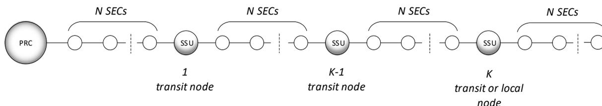
Figure 5.5: Synchronization Network Reference Chain adapted from ITU-T Rec G.803
