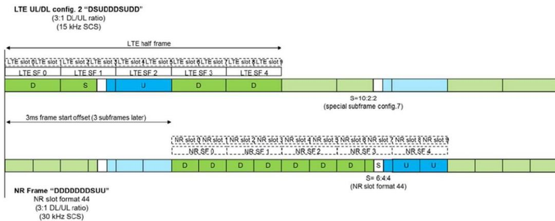
**Figure 4: Variant 2 - Synchronised operation of 5G-NR ("DDDDDDDSUU" frame) and LTE-TDD ("DSUDD" frame)**
